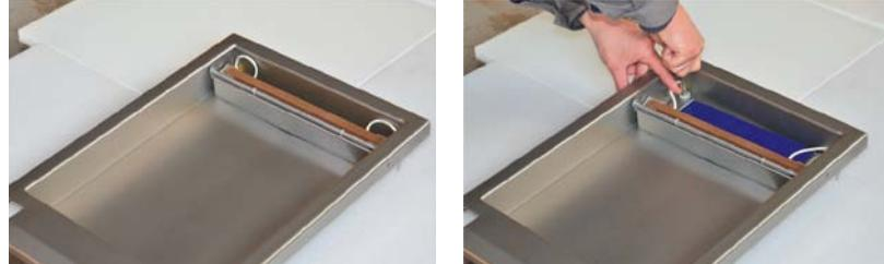
1. Disconnect the cable from the pin, then pick the complete sealing bar up from the vacuum chamber.
