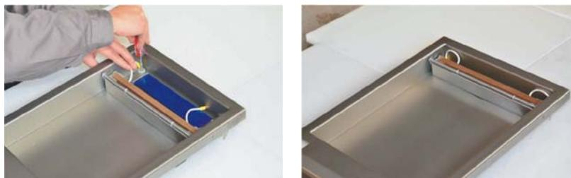
12. Connect the cable of the complete sealing bar to the pin, then put the sealing bar back in the vacuum chamber to complete the installation.
