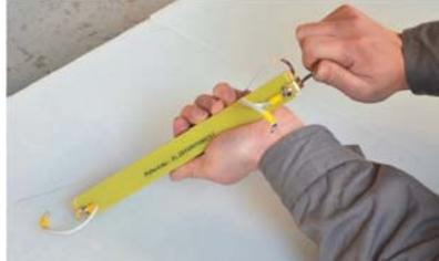
5. Put one side of a new heating wire into the fastener groove and tighten it with the Allen Key.
