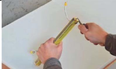
6. Put the other side of the heating wire into the other side fastener groove, then screw it with the Allen Key.
