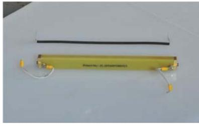
4. Remove the forcing screws from the two sides of the sealing bar with an Allen Key, then remove the heating wire.
