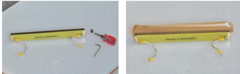
8. Take the new sealing tape at a proper length and stick it on the heating wire.
